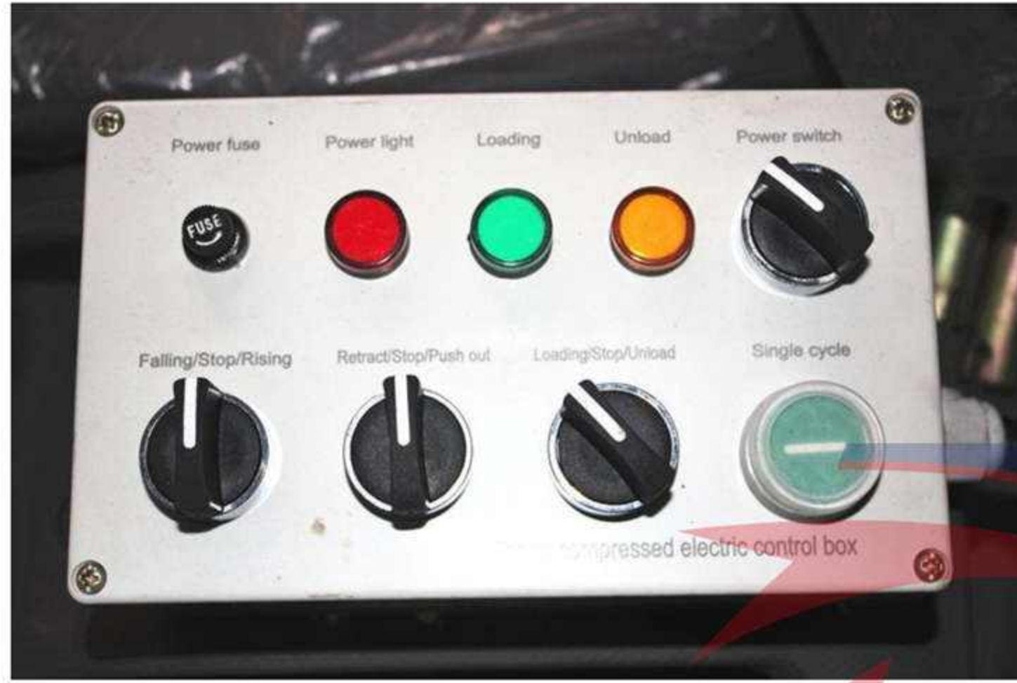
Main Control Box
